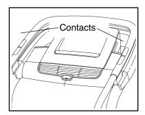
To measure your heart rate, stand on the foot rails and hold the pulse bar with your palms on the metal contacts; avoid moving your hands. When your pulse is detected, your heart rate will be shown. For the most accurate heart rate reading, continue to hold the contacts for about 15 seconds.
